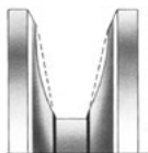
Worn Groove Sidewalls
