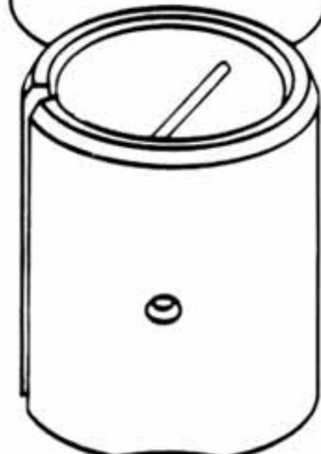
Internal Tension Bush (EG) with closed internal grease groove pattern and lubrication holes for radial lubrication application
