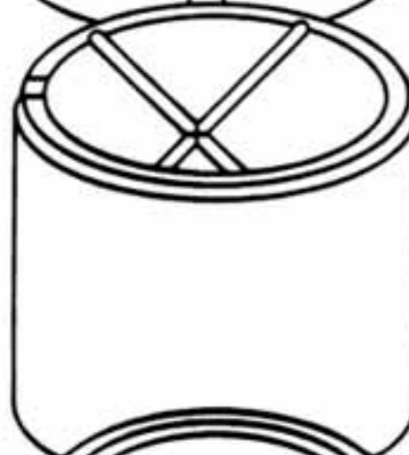
Internal Tension Bush (EG) with open "X" pattern grease grooves to permit flange sided lubrication
