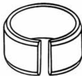
Internal Tension Bush (EG) with outside chamfers at both ends to facilitate automated assembly
