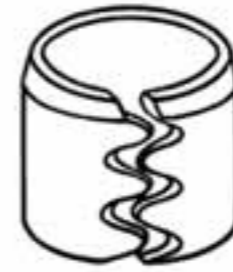
Internal Tension Bush (EW) with wavy slot for use on dynamic applications designed to distribute peak loads in the area of the slot
