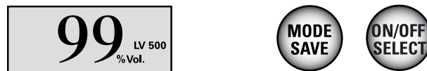
Fig. 22. Lubricator On. For an additional discharge, press both buttons at the same time and hold them down.
